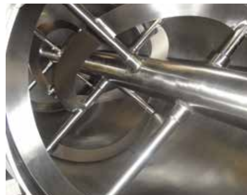
304L / 316L stainless-steel internal polishing
