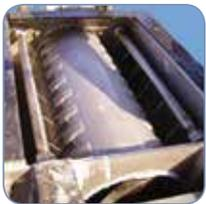
Outlet Compaction Section with Washing System (Option)
