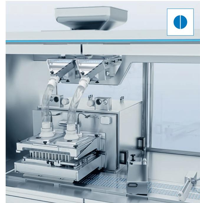
The **SimTap 4 feeder** feeds a wide variety of solid product shapes into the film pockets reliably, gently and precisely. A brush-in box can be attached to the basic module of the SimTap 4 in just a few steps. This means that two feeding principles can be implemented with one basic module – for particularly economical and efficient packaging.
