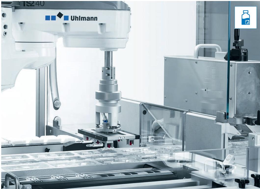
The **LiPro feeder** inserts vials, cartridges and ampoules into the blister pockets with high performance and optimal product protection.
