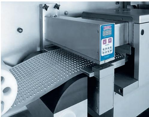
**VisioScan** detects film damage from as little as 10 µm and thus offers the best protection from invisible packaging defects.
