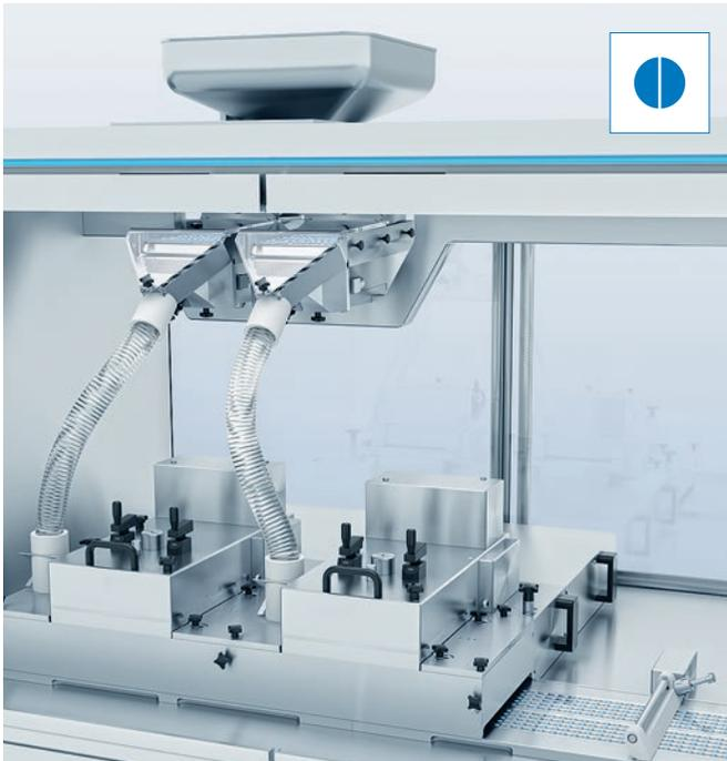
The **brush-in feeder** is suitable for thermoforming foils and can be used on both continuous and intermittent blister machines.
