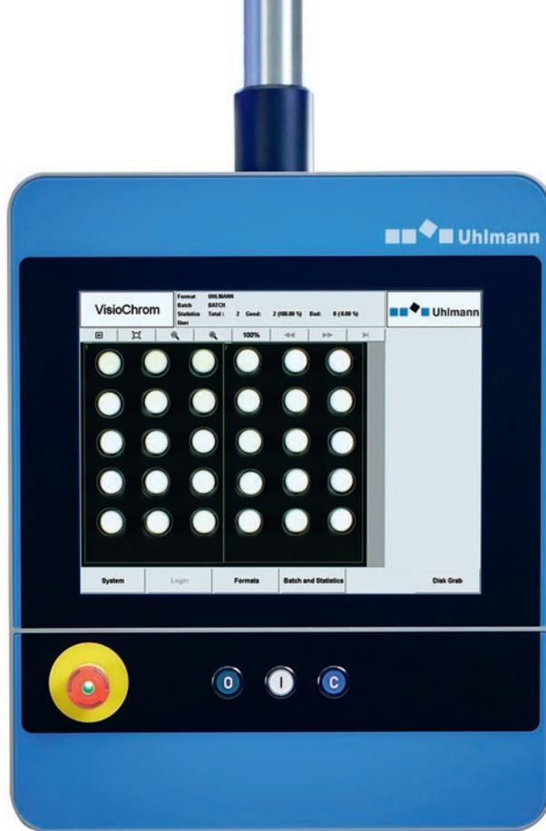
The color inspection system **VisioChrom** checks presence, position and color fastness and inspects up to 2,000 products per cycle.
