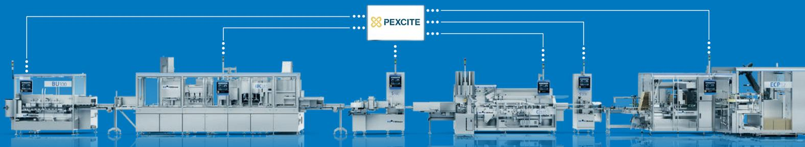
The Uhlmann proprietary software platform Pexcite networks all Uhlmann systems and equipment in the packaging of pharmaceuticals – for greater transparency and maximum pharmaceutical safety.
