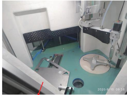
**The design of air flow direction is beneficial to maintaining the sample temperature on the plate rack in the pipe lifting area at  $-140^{\circ}\text{C}$  or below**
