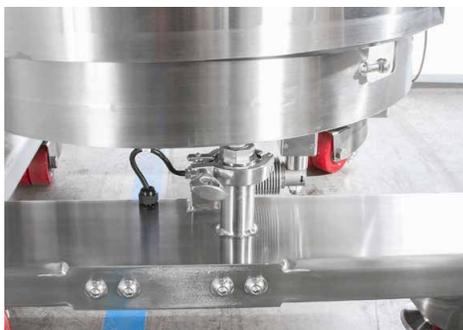
Figure 10. Load cells.
