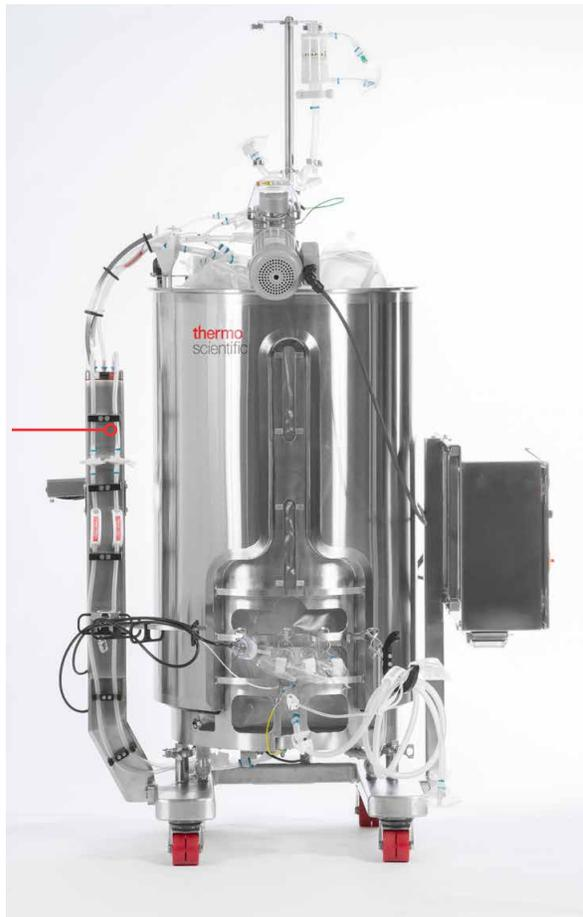
Figure 11. Tubing and cable management tree.
