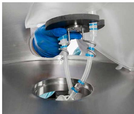
Figure 6. Sparge line support.
