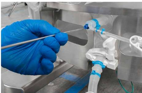
Figure 9. S.U.B. temperature sample port.
