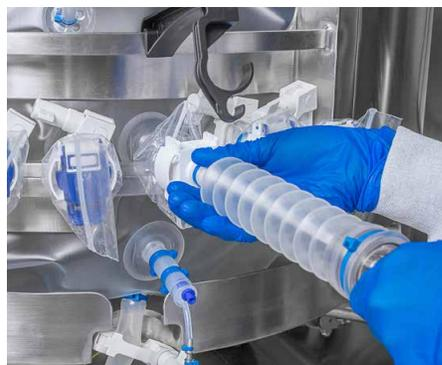
Figure 5. Bioreactor probe assembly.
