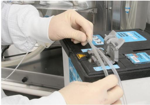
**Figure 3.82. Tubing welder.**
