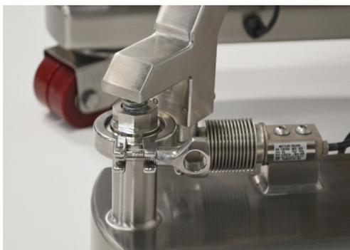
Figure 1.14. Load cell location.
