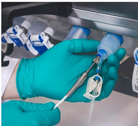
Figure 3.58. Inserting the RTD.
