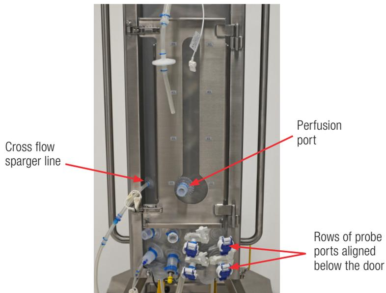
Figure 3.24. Door shut, with lines and ports aligned in cutouts.
