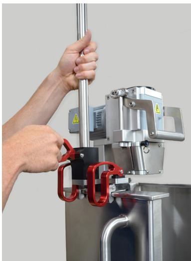
**Figure 3.13. Securing the exhaust vent filter to the holder.**
