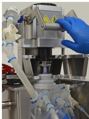
Figure 3.12. Pulling down on BPC lift lever and locking mechanism.
