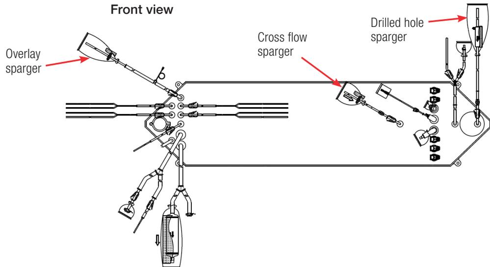
Figure 3.77. 500 L DynaDrive S.U.B. BPC spargers.
