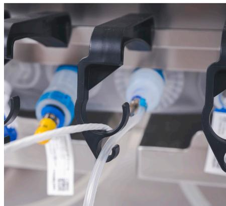
Figure 3.59. RTD placed in a probe clip.
