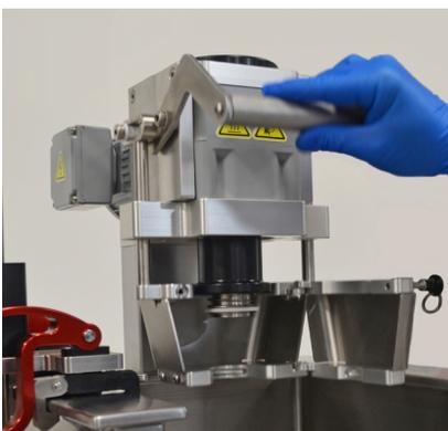
Figure 3.10. Raising BPC lift mechanism lever.
