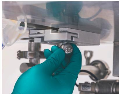
**Figure 3.46. Pushing the metal pin up to lock the gate.**
