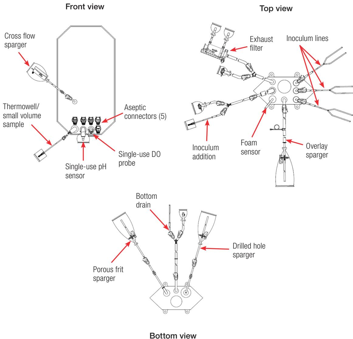
Figure 4.12. Front, top, and bottom views of 50 L DynaDrive S.U.B. BPC without ATF.
