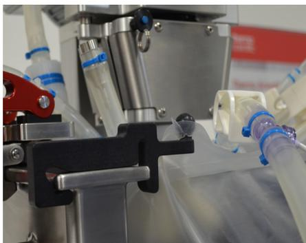
Figure 3.16. Black top tab holder with BPC tab attached.
