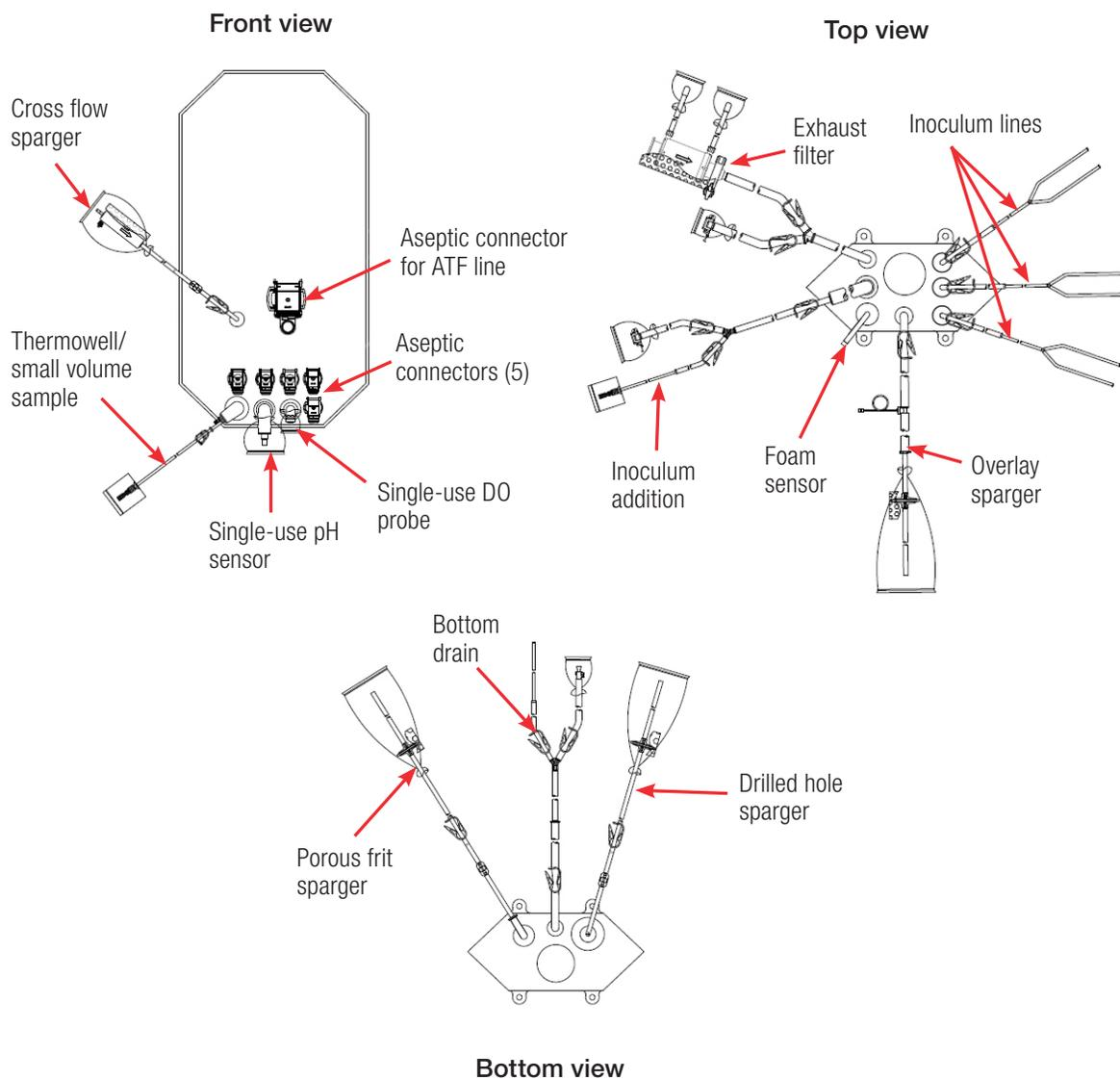
Figure 4.11. Front, top, and bottom views of 50 L DynaDrive S.U.B. BPC with ATF.
