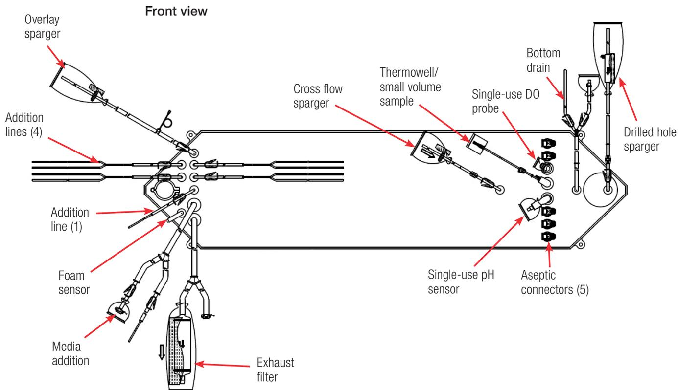
Figure 4.13. Front, top, and bottom views of 500 L DynaDrive S.U.B. BPC.
