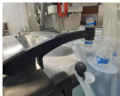
Figure 1.18. 500 L foam probe holder.
