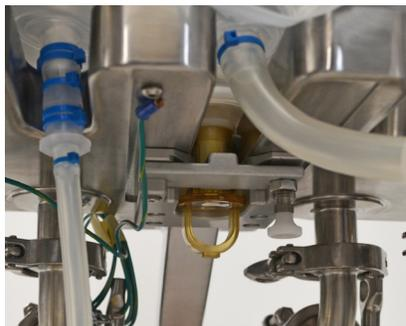
**Figure 3.21.** Positioning loop locked in place.
