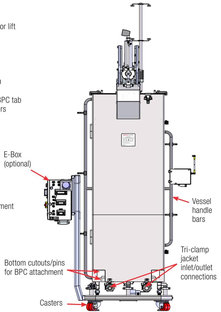
Figure 1.5. Back view of 500 L DynaDrive S.U.B. (with optional E-Box).
