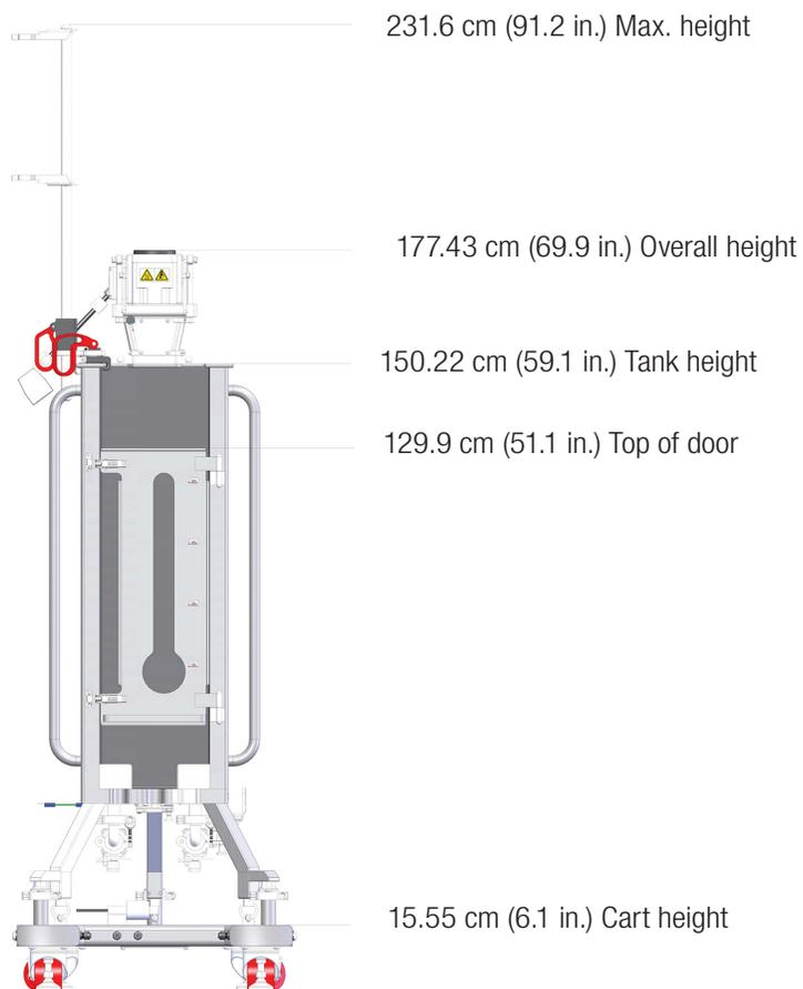
Figure 4.5. Dimensions of 50 L DynaDrive S.U.B. without optional E-Box (front view).
