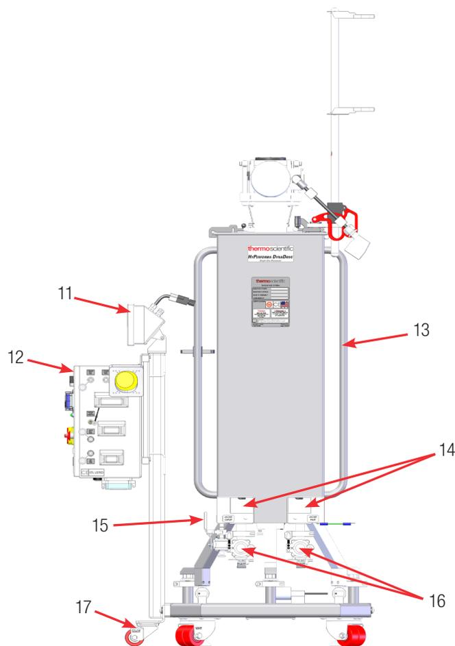
Figure 4.2. Back view of 50 L DynaDrive S.U.B. (with optional E-Box).
