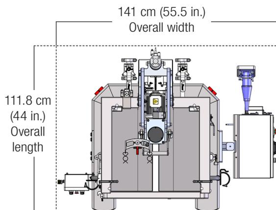
Figure 4.8. Dimensions of 500 L DynaDrive S.U.B. with optional E-Box (top view).
