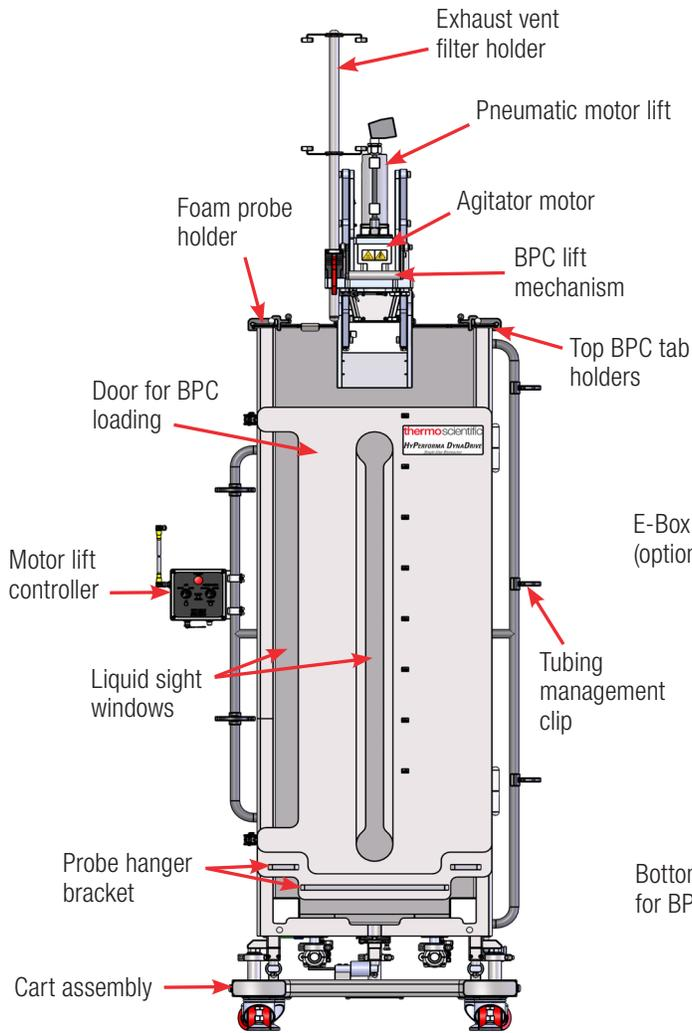
Figure 1.4. Front view of 500 L DynaDrive S.U.B. (without optional E-Box).
