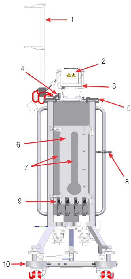
Figure 4.1. Front view of 50 L DynaDrive S.U.B. (without optional E-Box).
