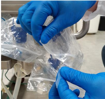
Figure 3.64. Pulling the tear strip.
