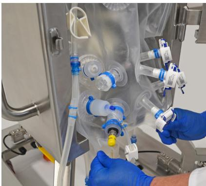
Figure 3.17. Pulling the bottom corners of the BPC to straighten out the sides.
