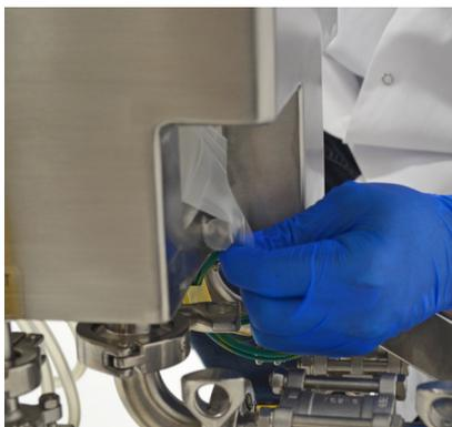
**Figure 3.23.** Pulling BPC bottom hanging tab toward bottom pin.
