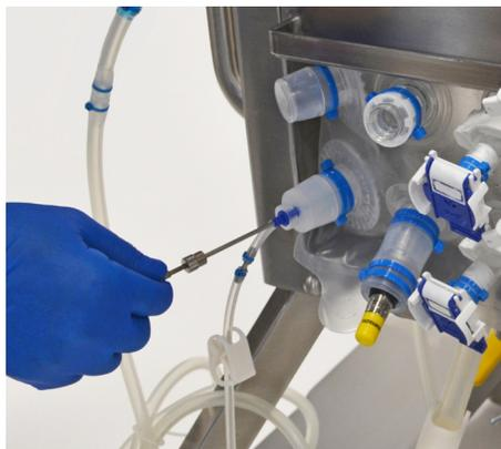
Figure 3.28. Inserting the RTD.
