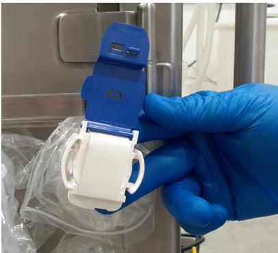
Figure 3.66. Opening the protective cover pull tab on the port.
