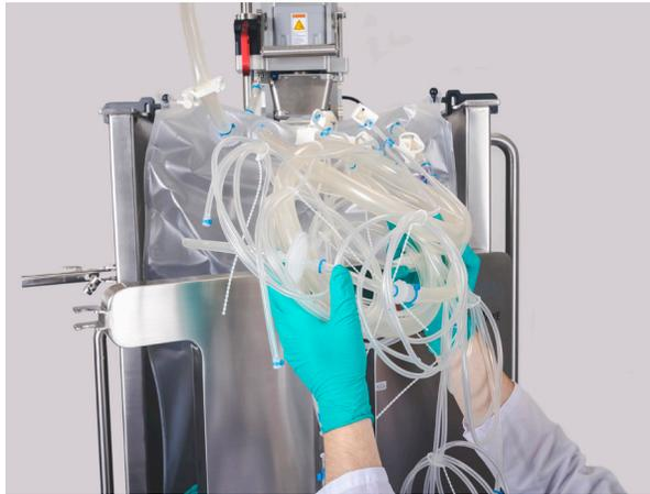
Figure 3.52. Lifting tubing line sets above the door while closing it.
