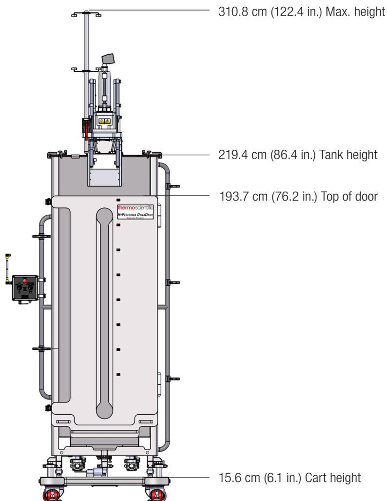
Figure 4.7. Dimensions of 500 L DynaDrive S.U.B. without optional E-Box (front view).
