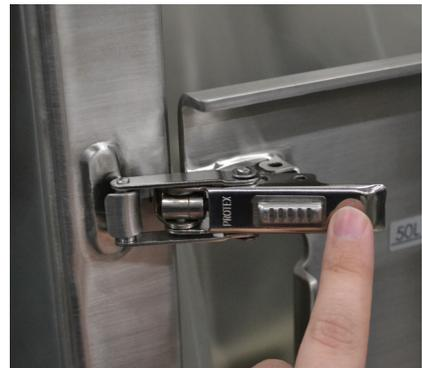
Figure 3.26. Closing door latch.
