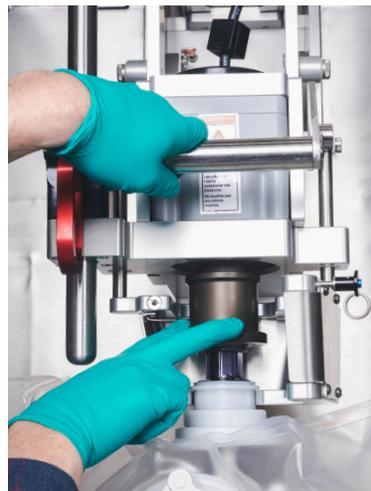
Figure 3.41. Pulling down on BPC lift lever and locking mechanism.
