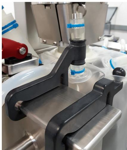
Figure 3.78. 50 L Foam probe in foam probe holder.
