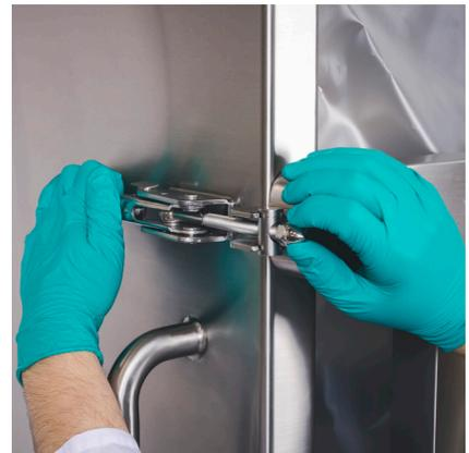
Figure 3.55. Securing the top door latch.
