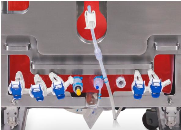
Figure 3.53. Probe port row aligned underneath the closed door (BPC shown filled).
