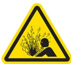
**WARNING:** The BPC is not rated as a pressure vessel. **DO NOT EXCEED** 34 mbar (0.5 psi) within the BPC or the system could fail, causing personal injury or damage to equipment. **DO NOT** leave the BPC unattended while inflating. Consult your sales representative for recommended air flow rates. The operating pressures at the level of the DynaDrive S.U.B. are of primary importance, and these values must be adhered to.
