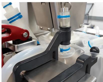
Figure 1.17. 50 L foam probe holder.
