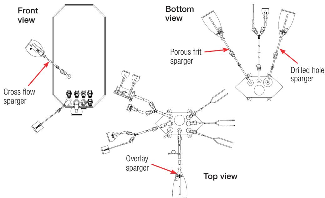
Figure 3.76. 50 L DynaDrive S.U.B. BPC spargers.
