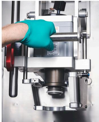
Figure 3.39. Raising BPC lift mechanism lever.
