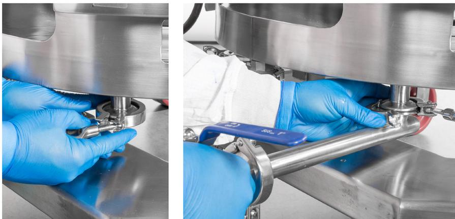
Figure 2.4. Removing the tri-clamp and attaching the fitting.
