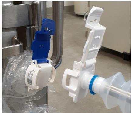
Figure 3.67. Aligning the connectors.
