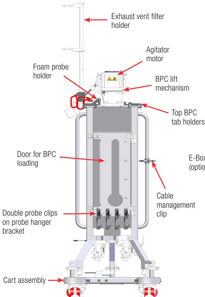
Figure 1.2. Front view of 50 L DynaDrive S.U.B. (without optional E-Box).
