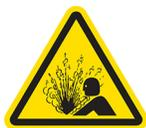
**WARNING:** The BPC is not rated as a pressure vessel. **DO NOT EXCEED** 34 mbar (0.5 psi) within the BPC or the system could fail, causing personal injury or damage to equipment. **DO NOT** leave the BPC unattended while inflating. Consult your sales representative for recommended air flow rates. The operating pressures at the level of the DynaDrive S.U.B. are of primary importance, and these values must be adhered to.
