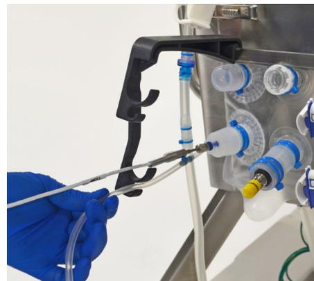
Figure 3.29. RTD placed in a double probe clip.
