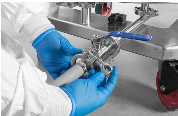
Figure 2.3. Attaching water jacket port using tri-clamp.
