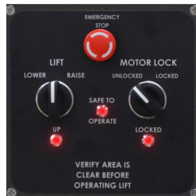
Figure 1.10. Red lights indicating lift is not raised, locked, or safe to operate.
