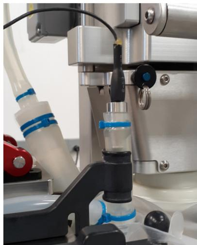
Figure 3.79. Foam sensor plugged into 50 L foam probe port.
