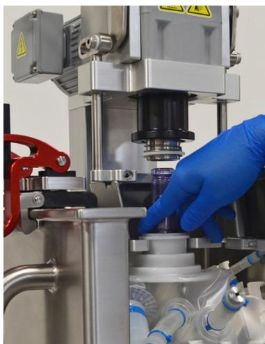
Figure 3.11. Aligning bearing hub with the bearing.
