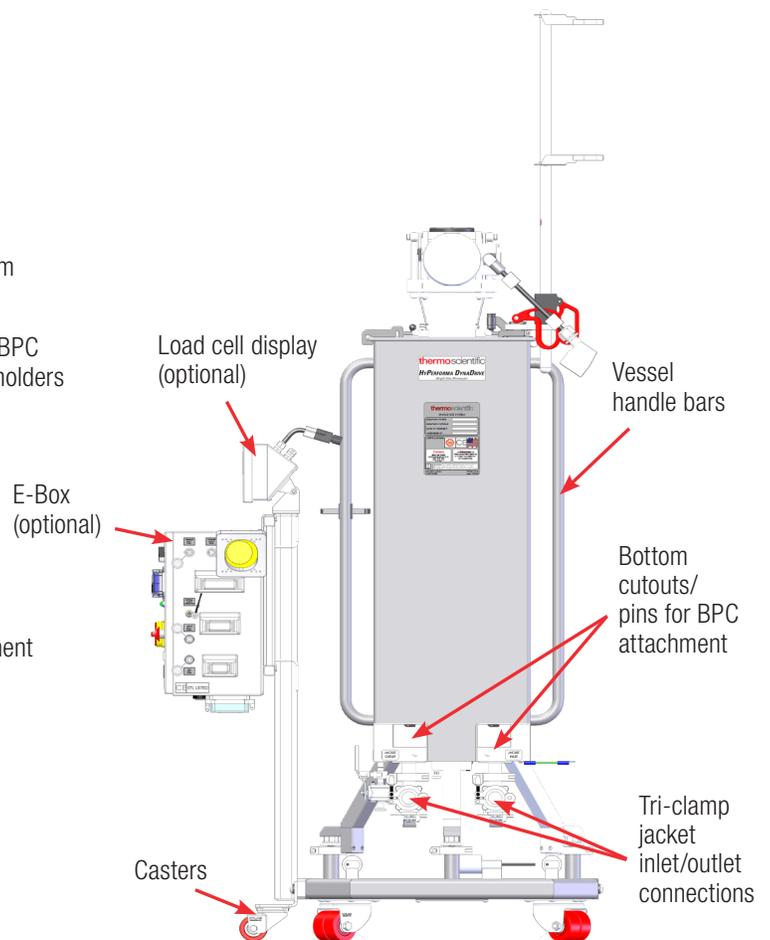
Figure 1.3. Back view of 50 L DynaDrive S.U.B. (with optional E-Box).
