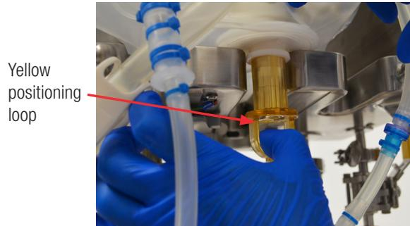
**Figure 3.18.** Yellow positioning loop aligned with the center cutout.
