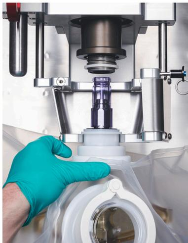
Figure 3.40. Aligning bearing hub with the bearing.
