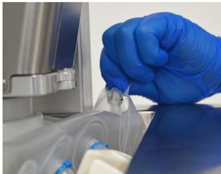
Figure 3.14. Pulling a top back hanging tab on the BPC towards the pin.
