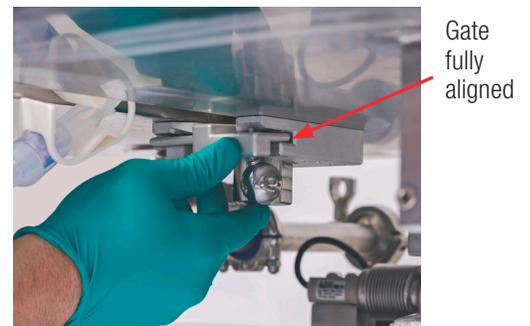
**Figure 3.45. Closing the gate completely.**
