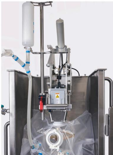
Figure 3.48. Pneumatic motor lift in lowest position.
