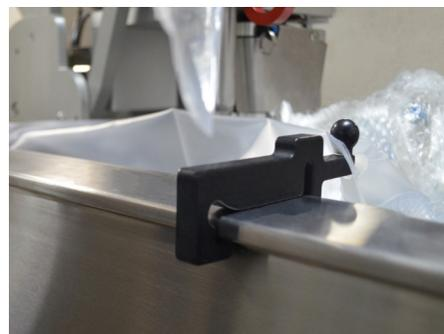
Figure 3.57. Black top tab holder with BPC tab attached.
