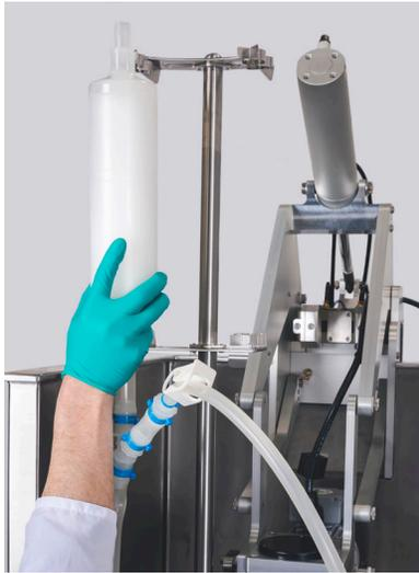
Figure 3.47. Securing the exhaust vent filter to the holder.
