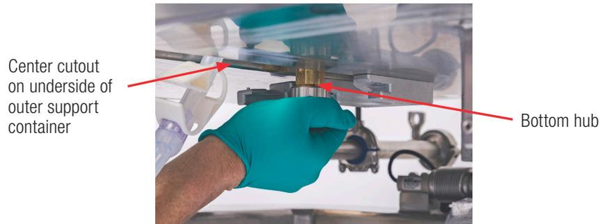
**Figure 3.43. Sliding the bottom hub into place in the front center cutout.**
