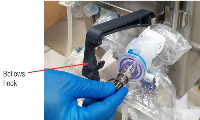
**Figure 3.72.** Lifting the probe before setting it into the bellows hook.
