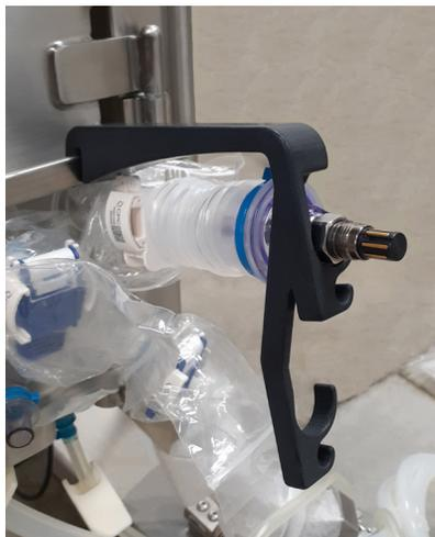
**Figure 3.73.** Inserted probe resting in bellows hook.
