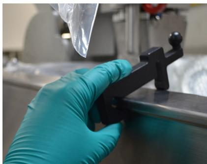
Figure 3.56. Placing the black top tab holders on the top front of tank.
