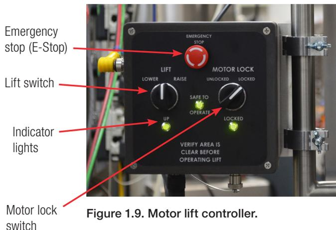
Figure 1.9. Motor lift controller.
