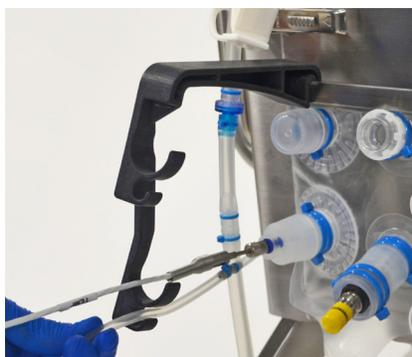
Figure 1.15. Double probe clip.
