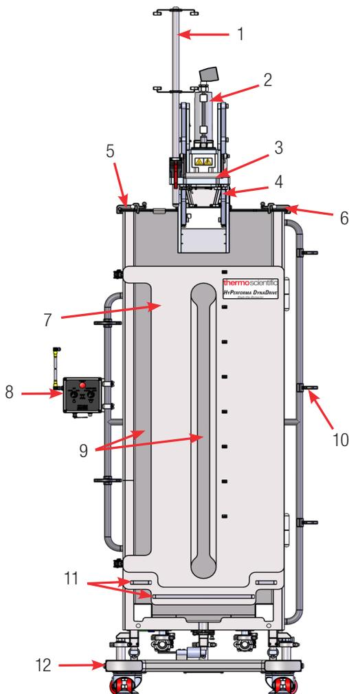
Figure 4.3. Front view of 500 L DynaDrive S.U.B. (without optional E-Box).
