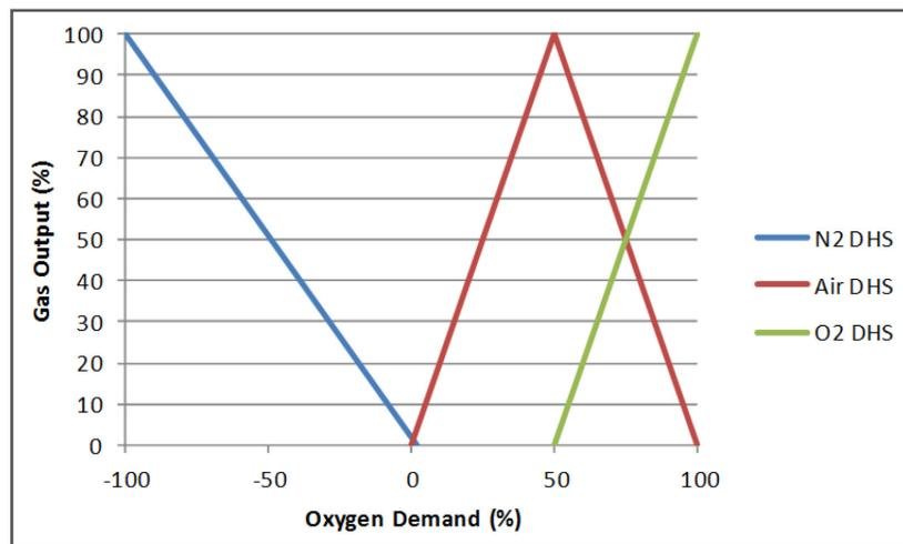
When progressing into higher positive DO control, the drilled hole sparger system is designed to maintain optimal oxygen delivery to carbon dioxide stripping rates. When drilled hole sparger flow rate limits are reached, supplant the sparger air flow with a steadily increasing ratio of oxygen to allow a higher degree of control.
