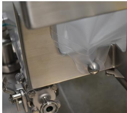
**Figure 3.51.** BPC bottom hanging tab attached to bottom pin.
