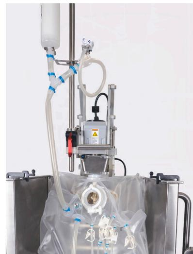
Figure 3.49. Pneumatic motor lift fully raised.
