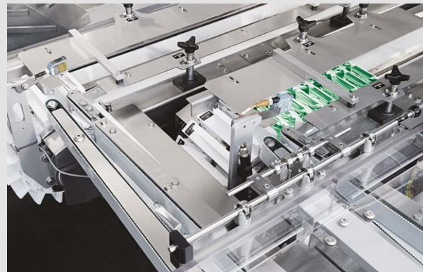
Double product infeed on edge and flat
