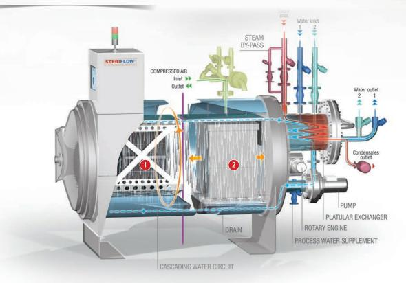
1 The Rotating Microflow is equiped with a stainless steel drum allowing product rotation during heat treatment. The basket containing the products rotates under heavy runoff. This improves heat transfer in the packaging while reducing cycle time.
