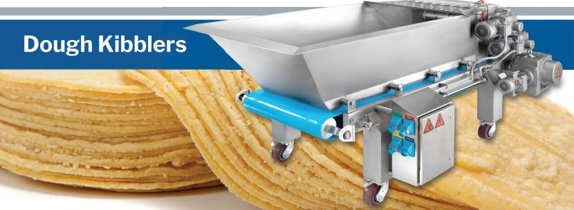
Shaffer® Dough Kibblers are used to break up dryer dough such as corn masa, cracker, and rotary moulded dough for feeding downstream processing equipment. The Kibbler can process an entire batch of dough by slowly conveying the dough mass through rotating tine cutters, discharging small usable sized (kibbled) dough chunks.
