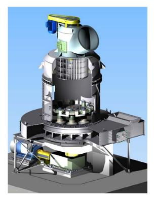
The roller mill, when equipped with a variable speed mill drive, can quickly be adjusted to accomodate changes in material hardness and feed size. This also allows the operator to match product rate with downstream process requirements, thereby reducing the operating and maintenance problems associated with frequent starts.
