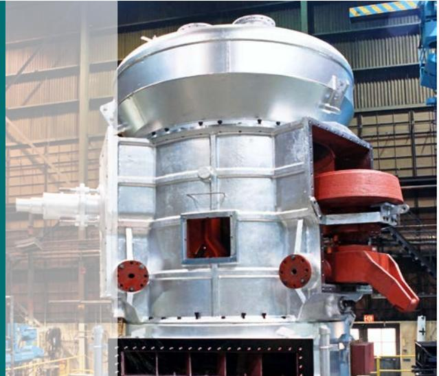
The Raymond® Bowl Mill with over 5,000 units in place worldwide is considered by many to be the finest machine available for pulverizing coal and pet coke as primary fuel for firing kilns, air heaters and other process equipment. It provides a safe, efficient means of uniformly pulverizing and drying these fuels.
