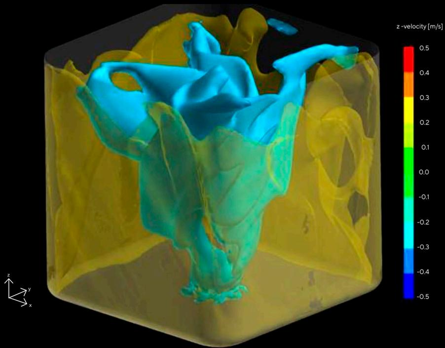
**Figure 5:** Simulation of Vertical Velocity in the Flexsafe® Pro Mixer (3D View)
