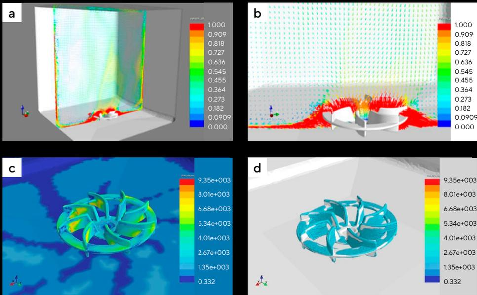
**Figure 6:** CFD Data for 200 L Flexsafe® Pro Mixer at 450 rpm.
