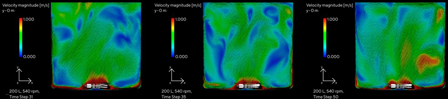
Note. Volume is 200 L and mixing speed is at 450 rpm. There are no permanent dead zones (blue).
