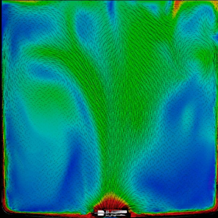
**Figure 2:** An Example of CFD Data Showing the Flow Pattern Inside a Cubical Mixer From the Side View
