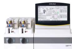
Ambr<sup>®</sup> 250 Modular system: comprising control module and bioreactor stations. Shown here with 2, the system is available with stations for up to 8 mini bioreactor vessels.
