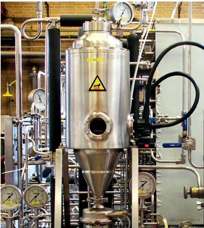
With a heating rate up to 600°C per second the infusion principle has proved to be a more gentle heat treatment process than injection UHT.
