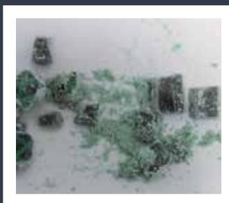
2 AFTER PRE-CUTTING IN A CUTTING MILL SM 300
