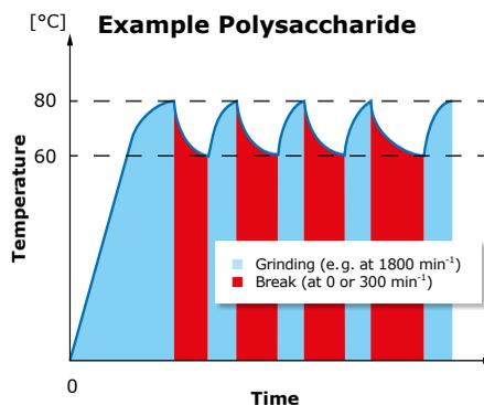
Fig. 4: Grinding of polysaccharide in a defined temperature range between 60°C and 80°C. Break times were automatically adjusted by the Emax software.
