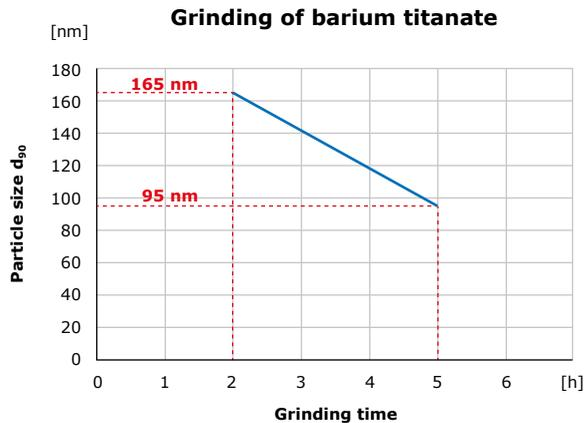
Fig. 2: Result of grinding 110 g barium titanate at  $500 \text{ min}^{-1}$  in the PM 100. After 2 hours of size reduction in 260 ml heptane with 0.5 mm grinding balls, the  $d_{90}$  value of the particle size distribution is 165 nm. By extending the grinding time to 5 h, the  $d_{90}$  value is reduced to 95 nm.
