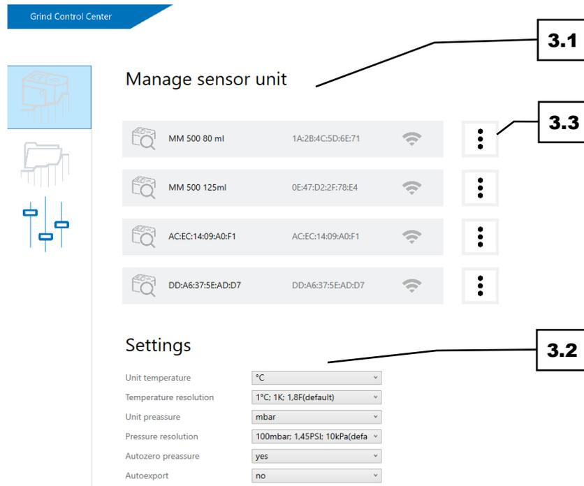
**Abb.17:** Manage sensor unit
