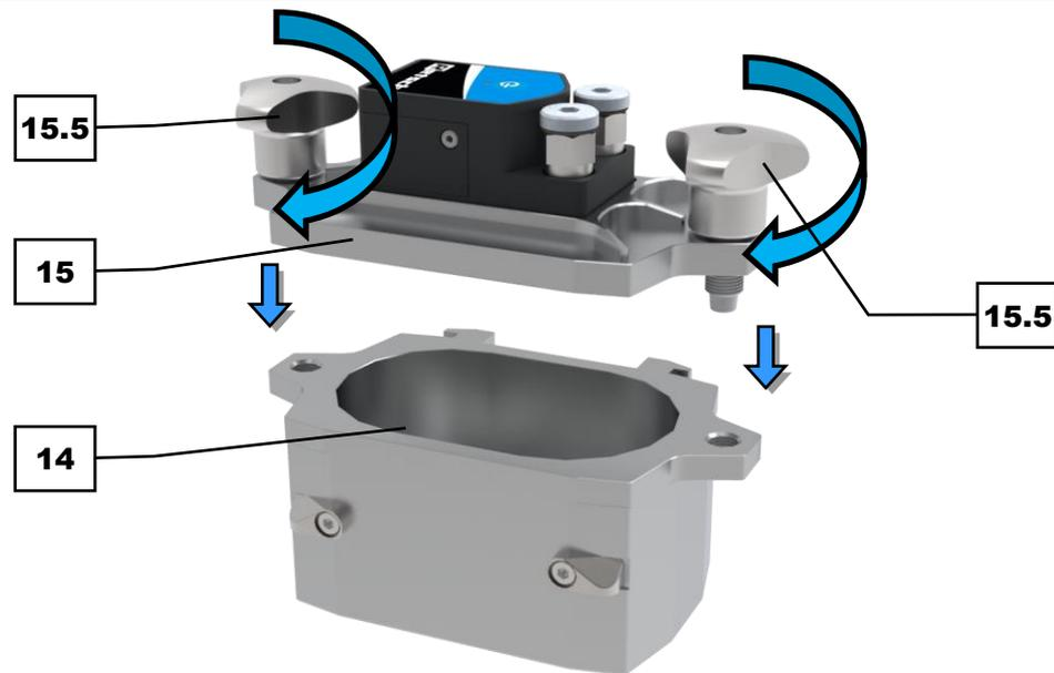
**Fig. 32:** Closing the grinding jar
