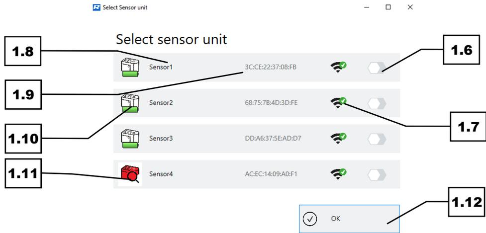
**Abb. 10:** Selecting the sensor unit
