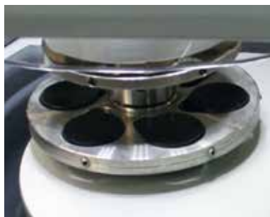
Central pressure requires levelled samples
