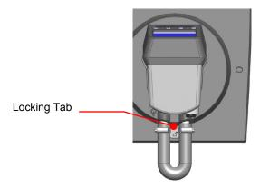
2. Rotate the Temperature Controller clockwise until it stops (about 0.75 inch / 1.9 cm).
