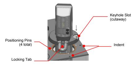
2. Gently rotate the Temperature Controller until it drops down on the Positioning Pins.
