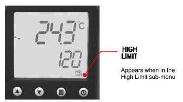
**To Access:** Press the key until HIGH LIMIT appears on the display.
