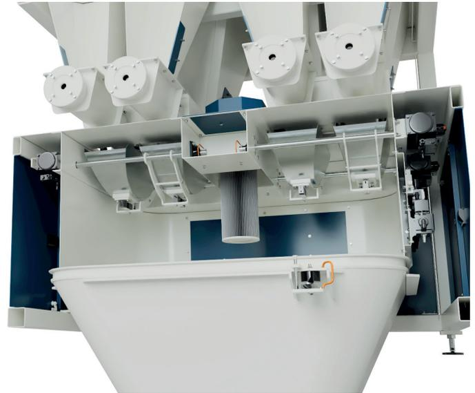
The Micro Dosing Unit (MDU) is a modular build high accuracy dosing system suitable for a wide range of different applications. It is also an easy expandable system in case needed. The MDU consists of a robust and hygienic designed base-frame made of steel box sections with the bin hoppers, dosing equipment and scales fully integrated.
