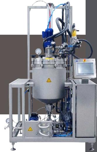
The OMVE batch cookers are modular build systems, used for various processes in the food industry. Depending on the configuration the system can be used for:
