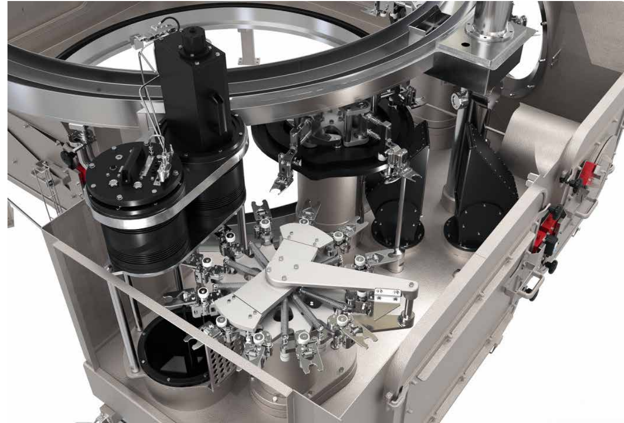
Sealing surfaces inspection in the Contipure AseptBloc
