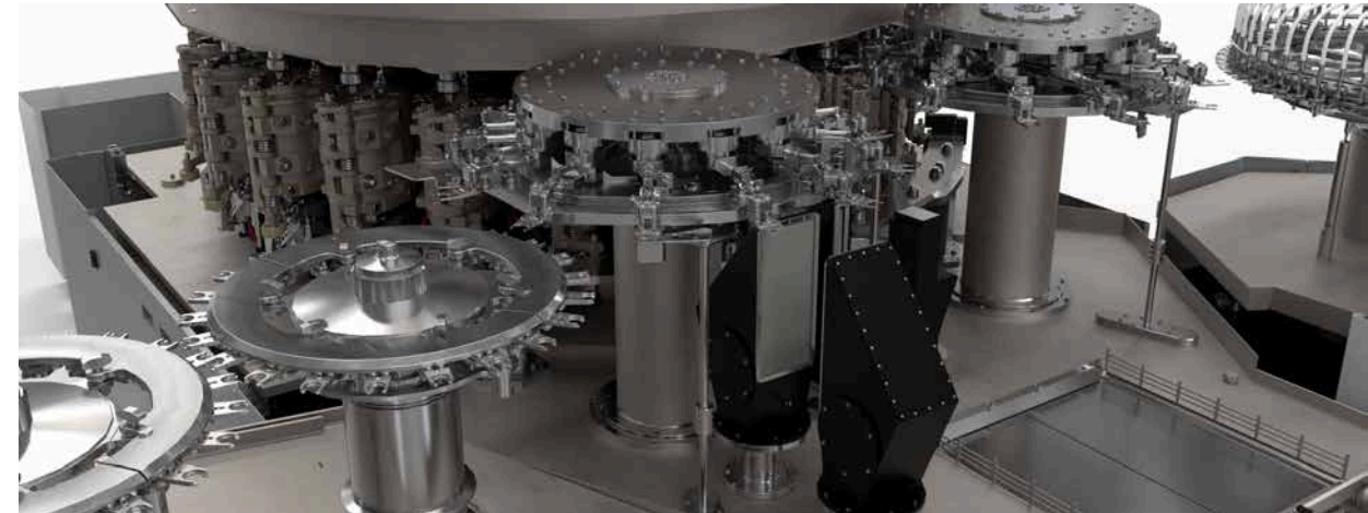
Contour and side-wall inspection in the Contipure AseptBloc
