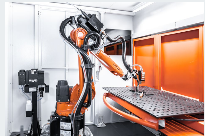
The KR CYBERTECH nano in a welding application
