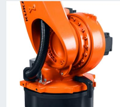
The space-saving and intelligently integrated cabling ensures that the KR CYBERTECH robots have maximum freedom of motion in any installation position.
