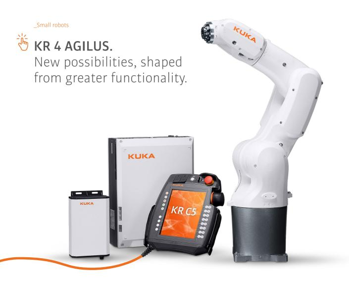
**Custom-tailored for maximum performance in production.** High performance in any installation position and with minimal space requirements – the KR 4 AGILUS will impress you with its compact design, long reach and high precision.
