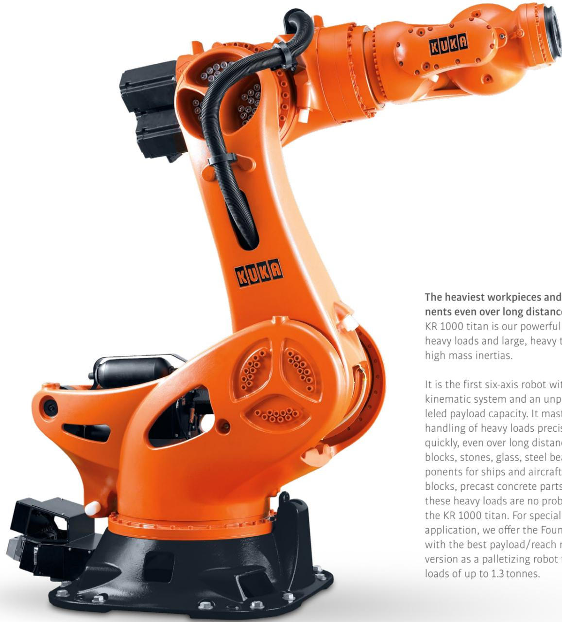
**The heaviest workpieces and components even over long distances.** The KR 1000 titan is our powerful robot for heavy loads and large, heavy tools with high mass inertias.
