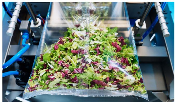
If a second product is fed into the GEWA washing machine via a second cutting machine or a second belt, for example different types of lettuce, the products are mixed at the same time by the HELICAL washing system during the washing process.
