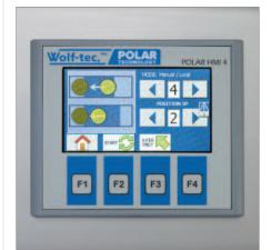
The PLC controller stores maceration programs for easy recall of all settings. With the push of a button, the roller clearance can be automatically adjusted.
