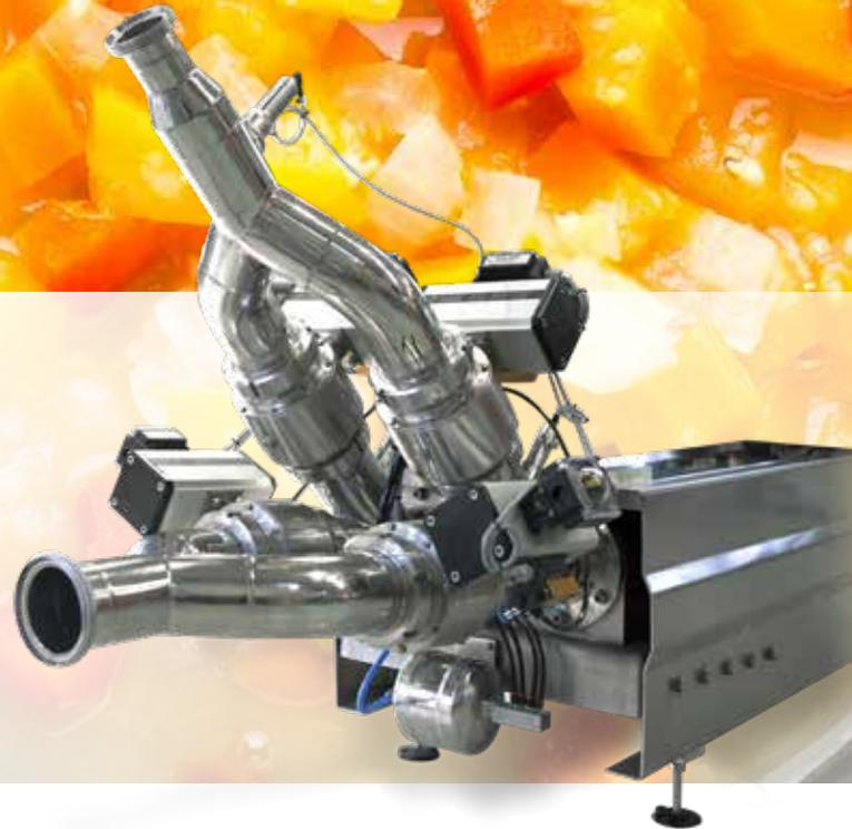
The Pumpideal™ has been specifically developed to treat products with large particulates up to 80mm (~3.15”) in size. Gentle product treatment is obtained at a maximum throughput of 10000 l/h (44 gpm) and an operating pressure of 15 bar (~218 psi).
