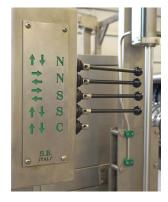
Hydraulically adjustable side banks simplify adjustments
