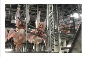
The Prime HM-1T Turkey Halving Machine automatically and effectively separates the front half from the saddle. The HM-1 can be adjusted to remove more rib bones or saddle to maximize yield. Working in conjunction with the BSC-Series Back Skin Cutter, The Halving Machine can be adjusted to completely cut front halves from the saddle or leave the front half hanging by the back skin to drop in a location downline from the halver.
