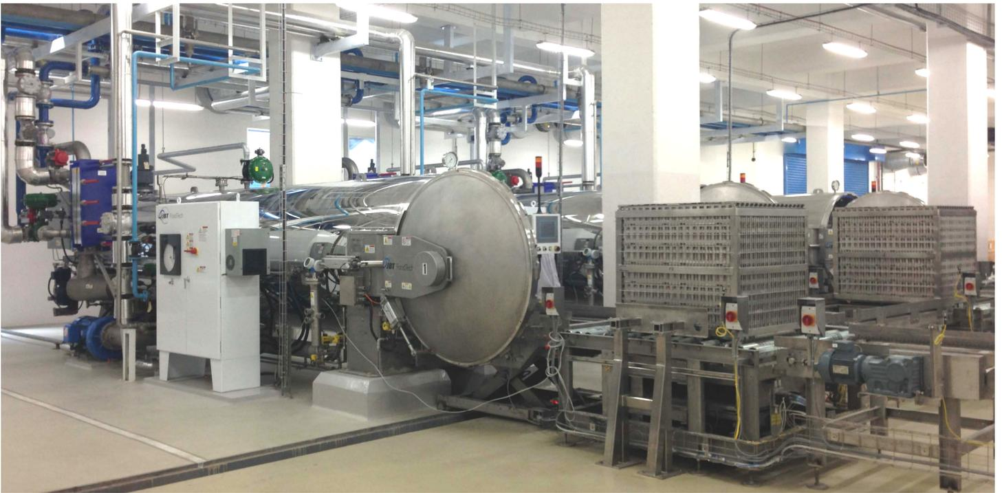
**Batch retorts** process product containers into baskets or crates. A steady flow of containers moves onto an accumulation table to a basket loader. The filled baskets form a train of product and are moved into a retort vessel for thermal processing. Once the cycle is complete, the baskets leave the retort vessel and are unloaded on a conveyor for further handling.
