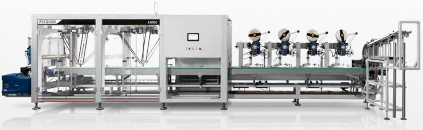
**CM** Platform encloses extremely innovative machines for the application of plastic lids on wet wipe packaging.
