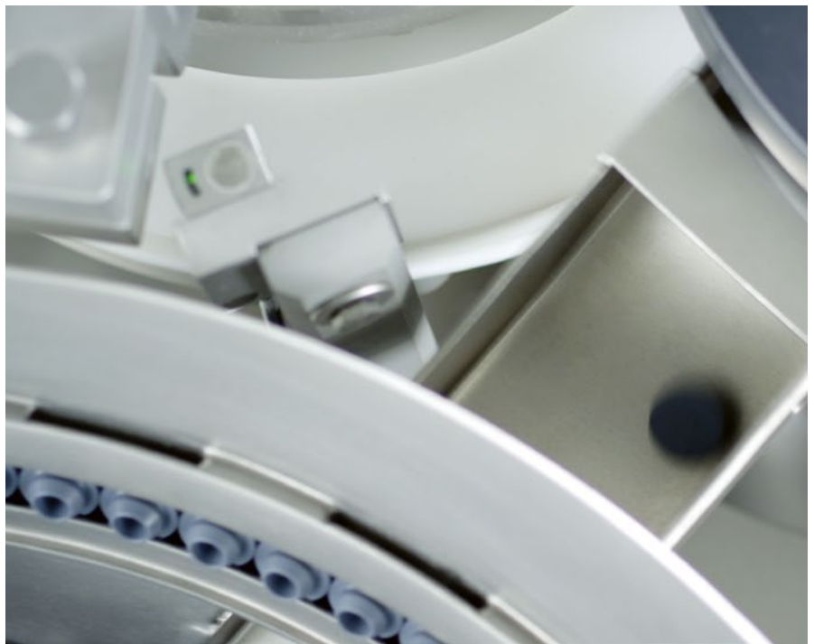
Stopper recovery in case of missing vial.
