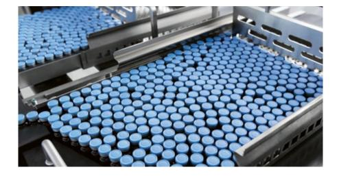
The VL series of tray loaders includes VL200 with compact dimensions and VL400-VL600 twin tray loaders. All models are designed to be installed in line with other machines.
