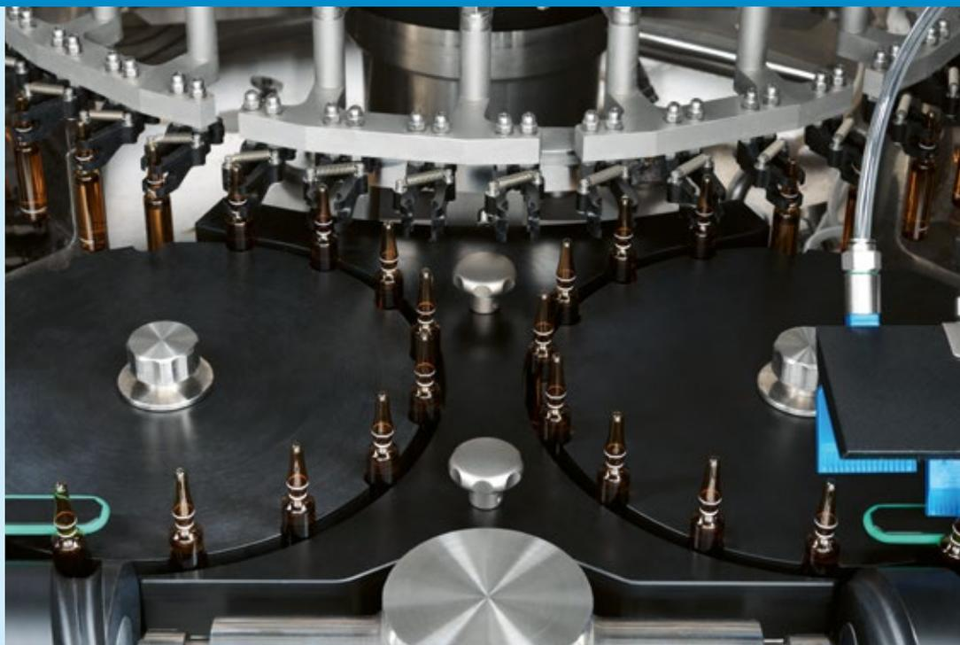
The containers are placed on a conveyor belt which keeps them compact during the loading phase. A scroll gently transfers the containers from the infeed belt to the transport starwheel where they are picked up by the pincers mounted on the central carousel.
