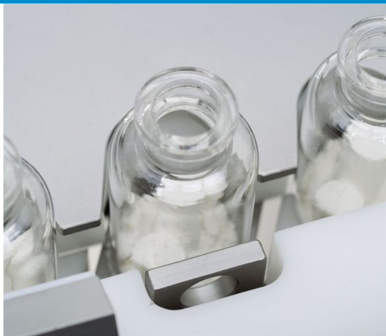
100% IPC gross weight sampling after dosing
