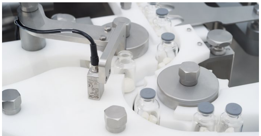
Vial rejection in case of missing stopper
