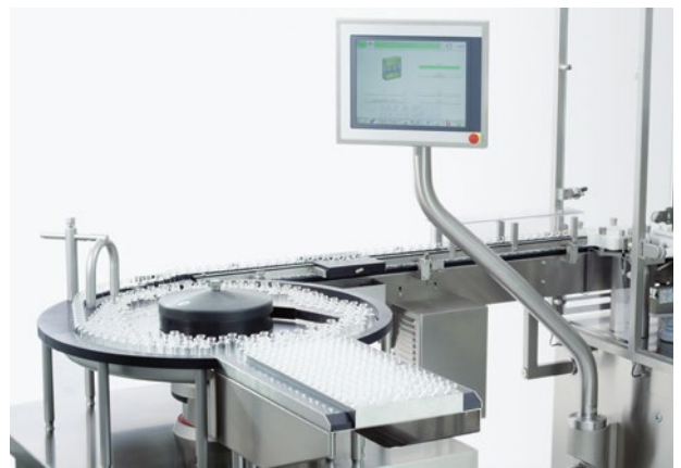
Machine configuration with upstream vial feeding table
