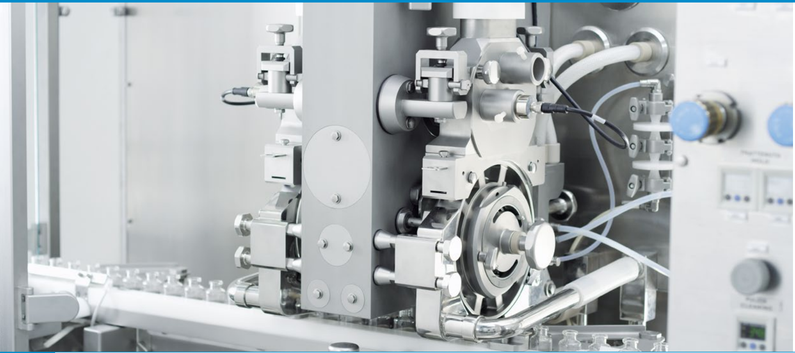
Powder dosing unit with two dosing discs
