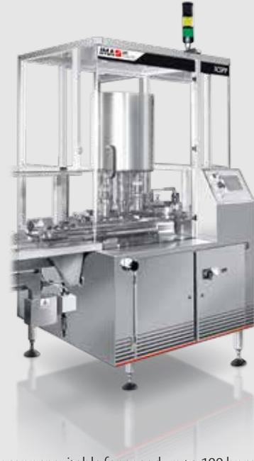
A 3 head rotary capper suitable for speed up to 100 bpm. Machine can handle round or irregular shaped containers, screw or press-on caps. The cap feeder is mounted on a simple electrically adjusted stand complete with an enclosure around the cap feeder for noise reduction, the capper turret is a powered adjustment to accommodate different height bottles.
