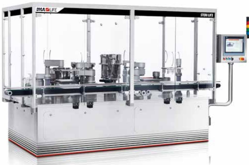
STERI LIF3 ROBOTIC ARMS OFFER REPEATABILITY WITH THE FLEXIBILITY TO EASILY CHANGE THE PROCESS OR THE TYPE OF CONTAINER BEING FILLED.
