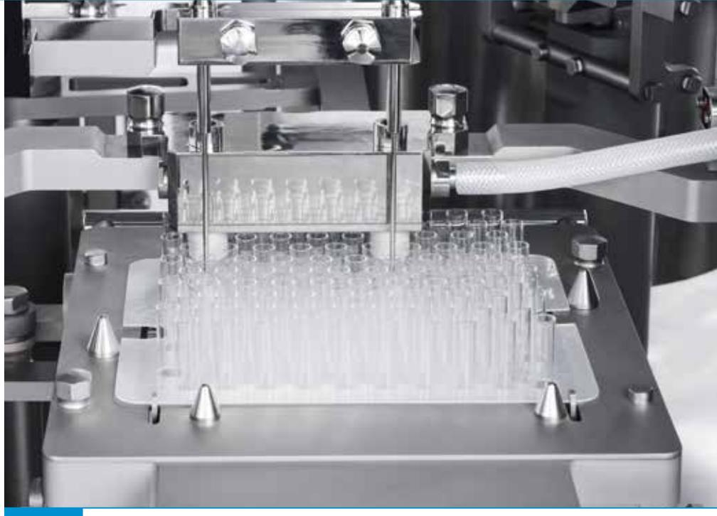
RTU cartridge filling and plugging
