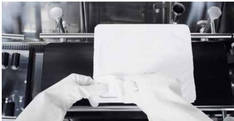
Manual de-lidding and linear removal under isolator
