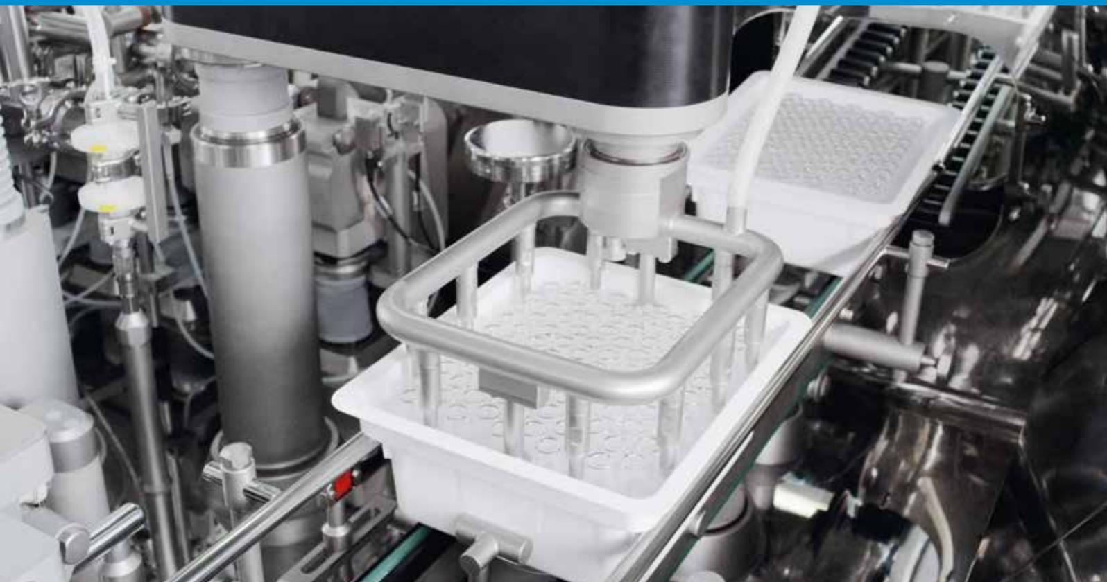
Sterifill RS Series automatic denesting at infeed
