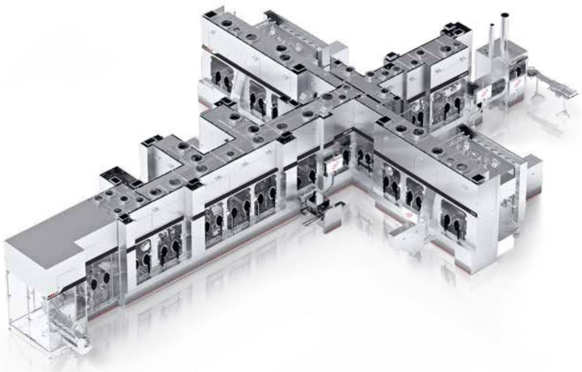
By embracing and adopting new robotic technologies throughout all production operations, from outer/inner bag opening to the stoppering station, INJECTA allows for a very smooth production process, drastically reducing human interventions and therefore cross-contamination risks.
