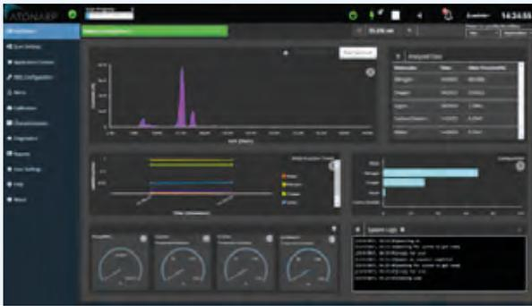
Typical Applications: end-point detection Water vapor, N<sub>2</sub>, CO<sub>2</sub>, He and O<sub>2</sub> detection and Si-Oil contamination detection.
