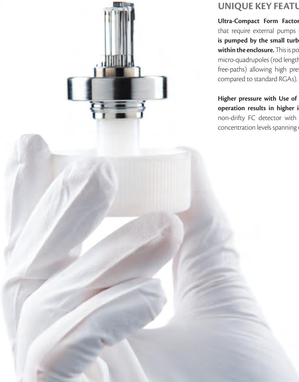
Quantitative and Accurate: QUANTUM is unique in its **ability to deliver highly accurate measurements in the order of sub-1%**. This unique advantage is made possible due to its innovative electronics and signal processing. Further, its operation allows calibration within the same pressure range against the gold standard Capacitance Diaphragm Gauge (CDG).
