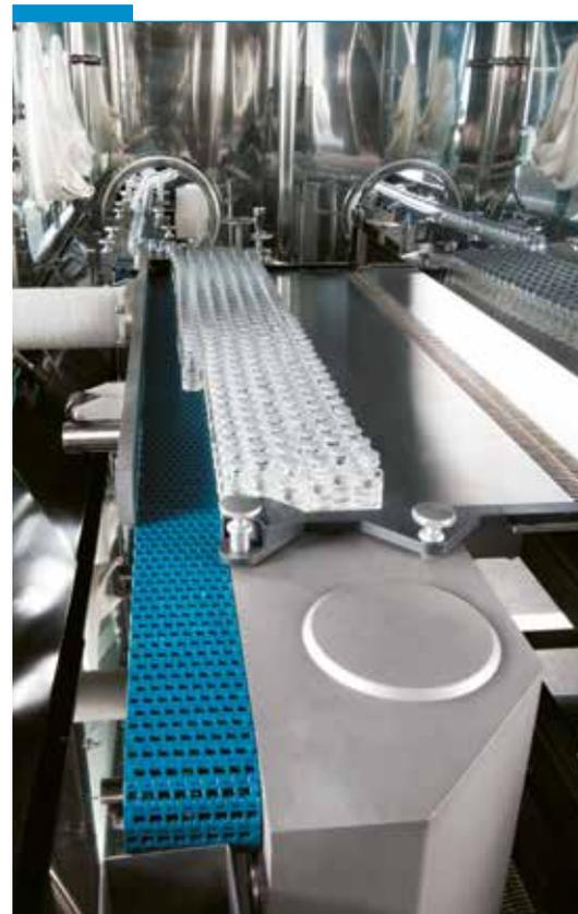
Pre-stoppered vial loading into freeze dryer
