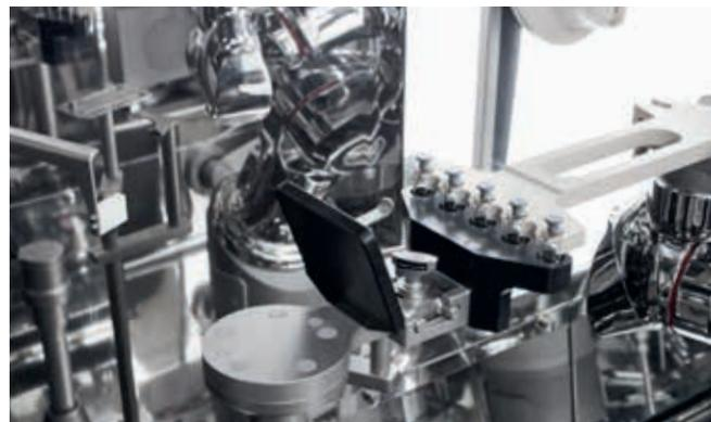
enhance process quality. A patented device eliminates the electrostatic charge in the nest for more accurate weighing. The handling system also minimises interference caused by airflow. Individual de-nested components are filled, check-weighed and immediately stoppered, reducing sterile drug exposure times. Weigh-cell block design allows for tolerance required to manage different RTU component formats.
