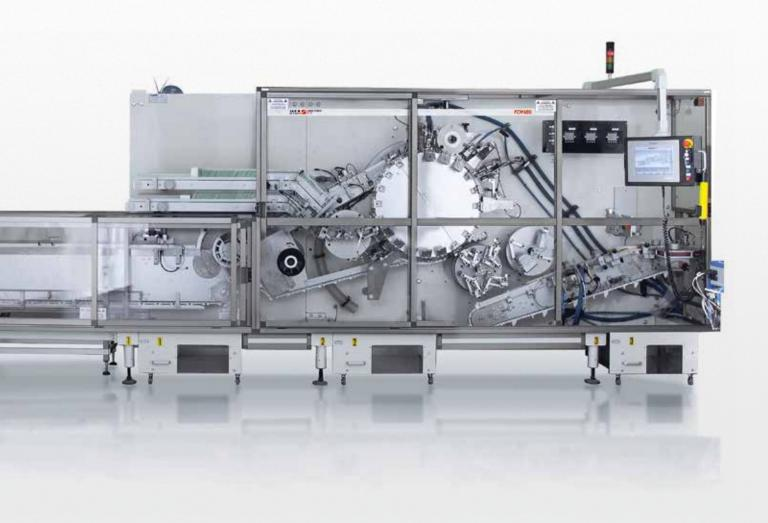
Continuous motion high-speed rotary cartoner for **flat blanks**, which ensure lower procurement costs compared to a pre-glued carton.
