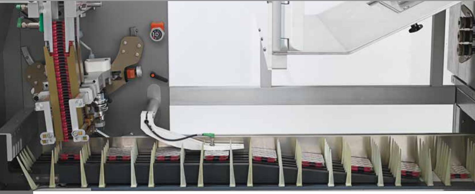
A COMPACT AND RELIABLE CONNECTION BETWEEN BLISTER MACHINE AND CARTONER WHILST RETAINING COMPLETE ACCESSIBILITY.
