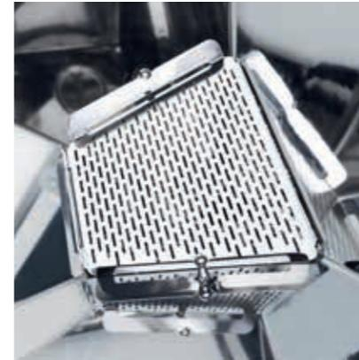
Different racks and baskets are available for optimal washing even of flexible hoses, drums, little containers and other components. When cleaning machine parts with a complex design, additional spray nozzles can be added to the washing basket, thereby increasing cleaning efficiency.
