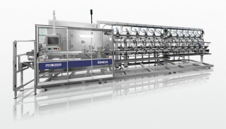
**GENESIS** is a length-fold wet wipes converting line that can handle from 6 to 12 pre-cut rolls with manual or automatic splice for maximum flexibility and easiness of use.
