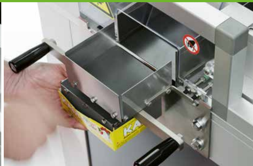
Semi-automatic tray formation and outfeed
