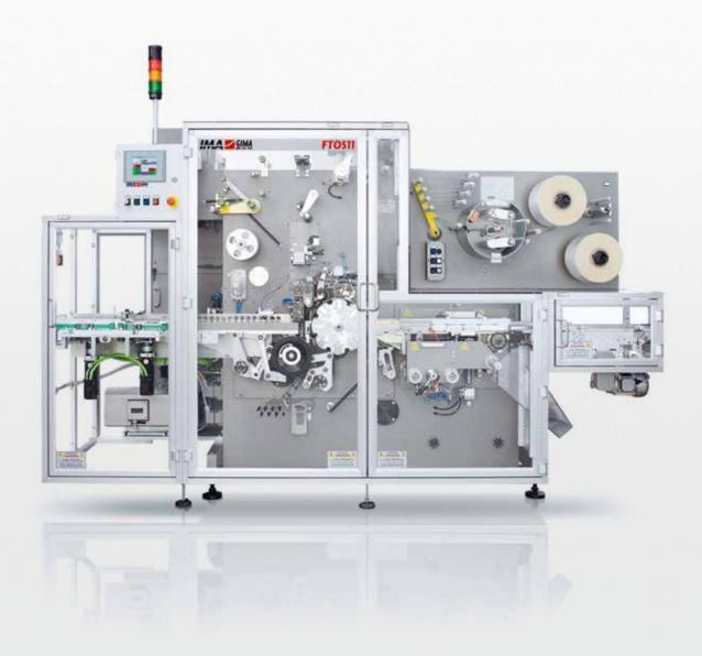
Ultra high-speed (**up to 500/min.**) overwrapping machine with continuous carton feeding system which prevents products from pushing against each other both at the start and at end the end of the line. Thanks to advanced technical solutions, such as the inline tear-tape unit, the double reel holder and the automatic film splicing, this machine ensures top quality appearance of packages.
