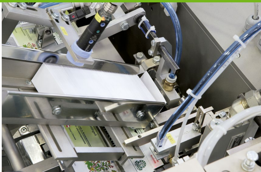
BEFORE CARTON CLOSING, AN OPTIONAL DEVICE CAN INSERT A PRE-FOLDED LEAFLET
