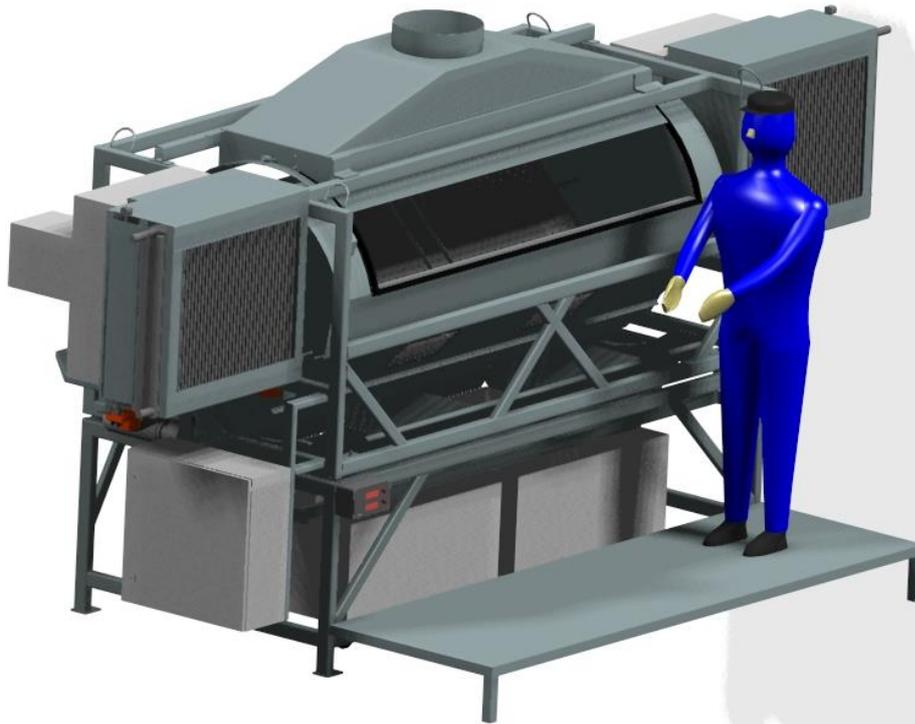
The heating can be done in several ways, the most simple way is to use Hot Water Heat Exchangers.
