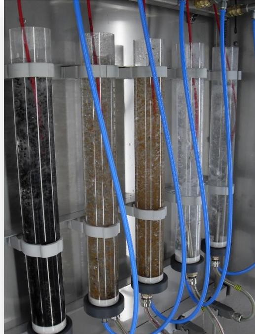
Each cylinder can run with its own day/night and temperature regime for testing several protocols at one run. We can also supply a “sophisticated” control system with logging to have more sight on the complete process.
